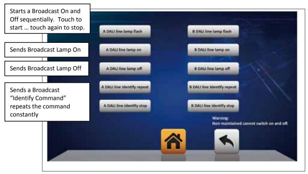
The "Identify Command" causes the fitting to flash its LED status indicator with the 6 bit structure of the physical Short Address as set In the device
