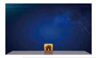
This is the opening screen and it will be displayed as soon as power is applied. While it is displayed the Application Controller is scanning the two DALI lines and establishing what is connected.
